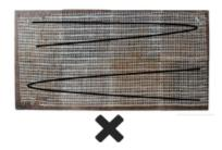
4. Repeat this process by adding glue to each subsequent piece and connecting it to the last. Be sure to leave a ½" expansion gap around the perimeter of the wall to allow for expansion and contraction of the wood with changes in temperature and humidity levels.
